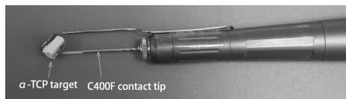
Fig 1. Compact Er:YAG laser ablation unit.
