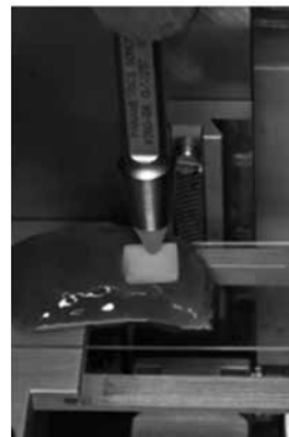
Fig.2 Set up of the bovine dentin and lever
